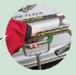
**Step One...**Squeeze handle up to release the hatch. Lower the bike rack.
