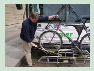
**Step Three...**Pull the support arm up and out and place it over the front bike tire. This arm locks the bike in place.
