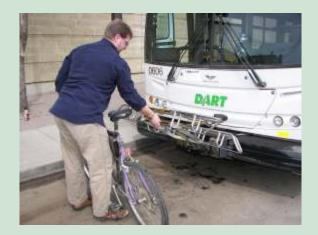
**Step Three...**If your bike was the last bike on the rack, squeeze the handle toward you and fold the rack back up against the bus.
